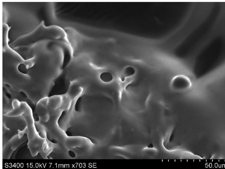
*Scanning electron microscopy (SEM) image of cellulose char produced in (a) open crucible and (b) crucible covered by a lid*
