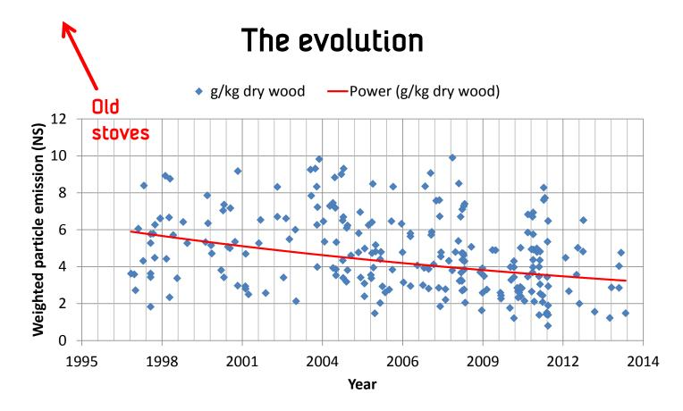
Weighted particle emission levels as a function of year or development degree
