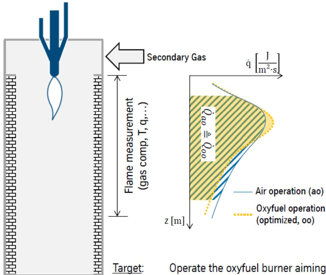
Target: Operate the oxyfuel burner aiming to achieve equal heat fluxes over a defined combustion chamber length
