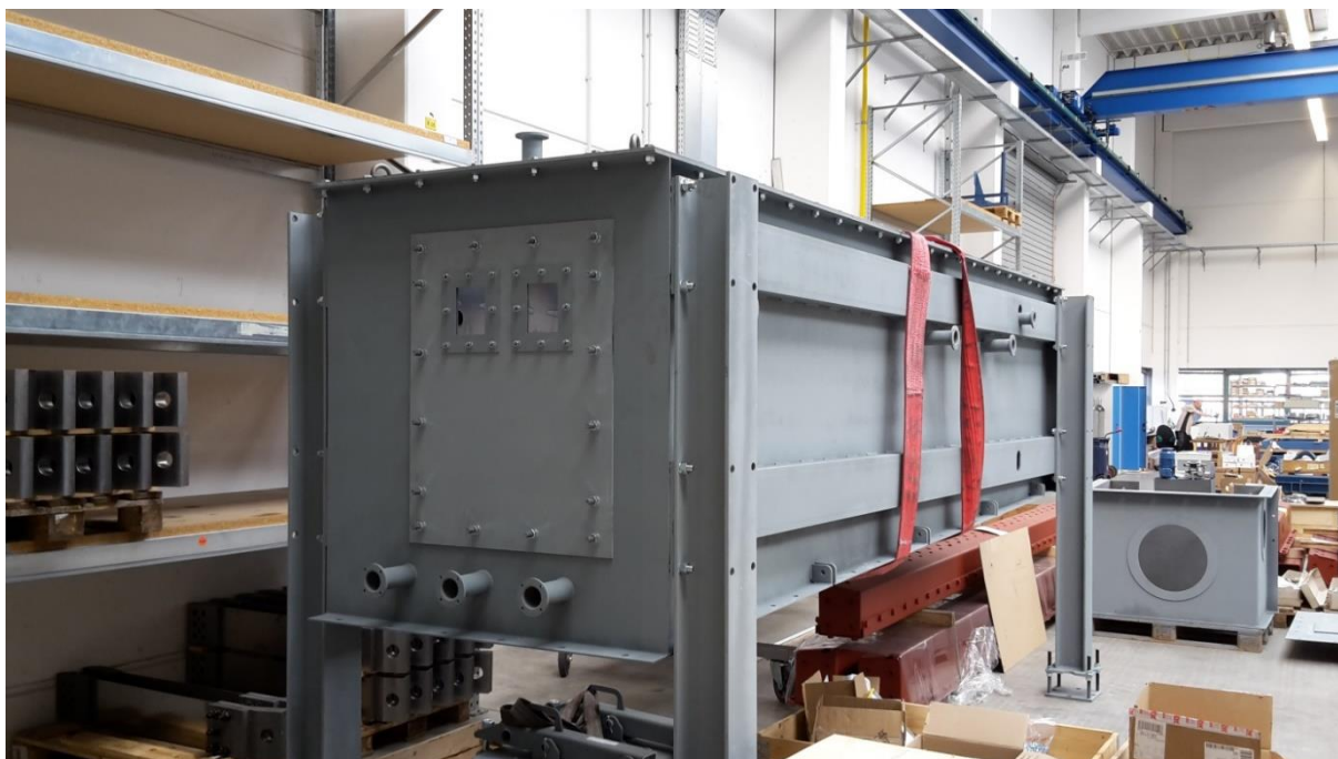
Figure 3.2: Oxyfuel clinker cooler prototype upper cooler housing pre-assembly.
