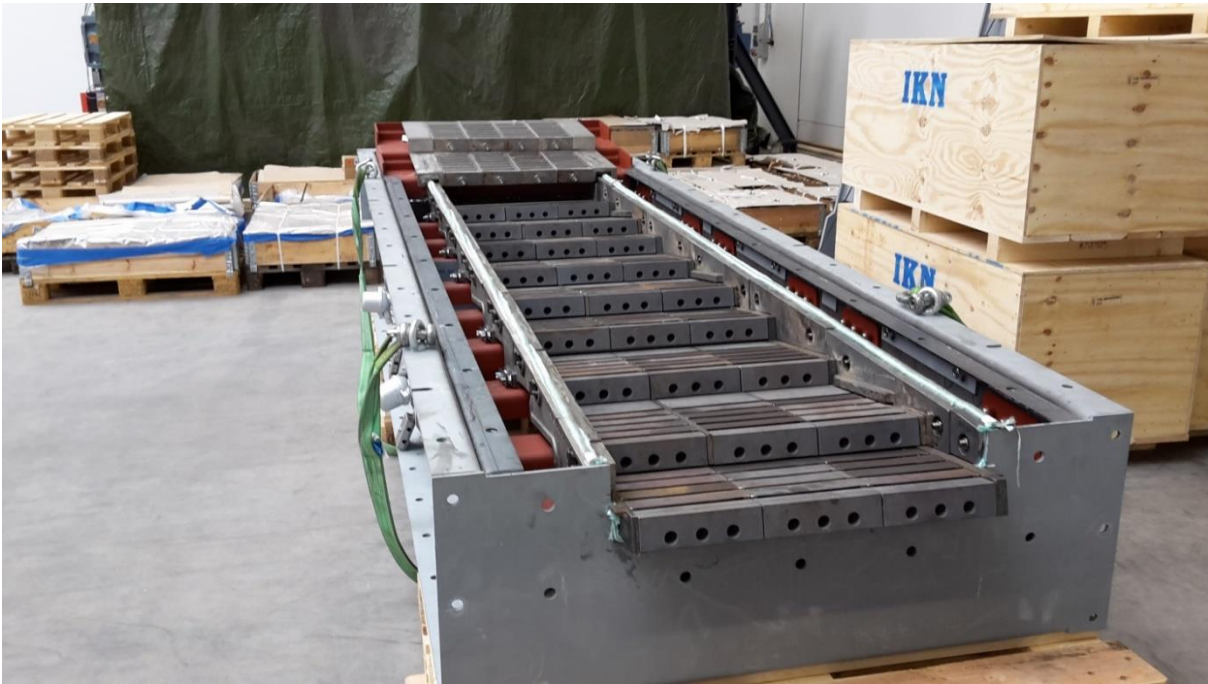
Figure 3.4: Oxyfuel clinker cooler prototype grate on lower cooler housing pre-assembled at IKN warehouse
