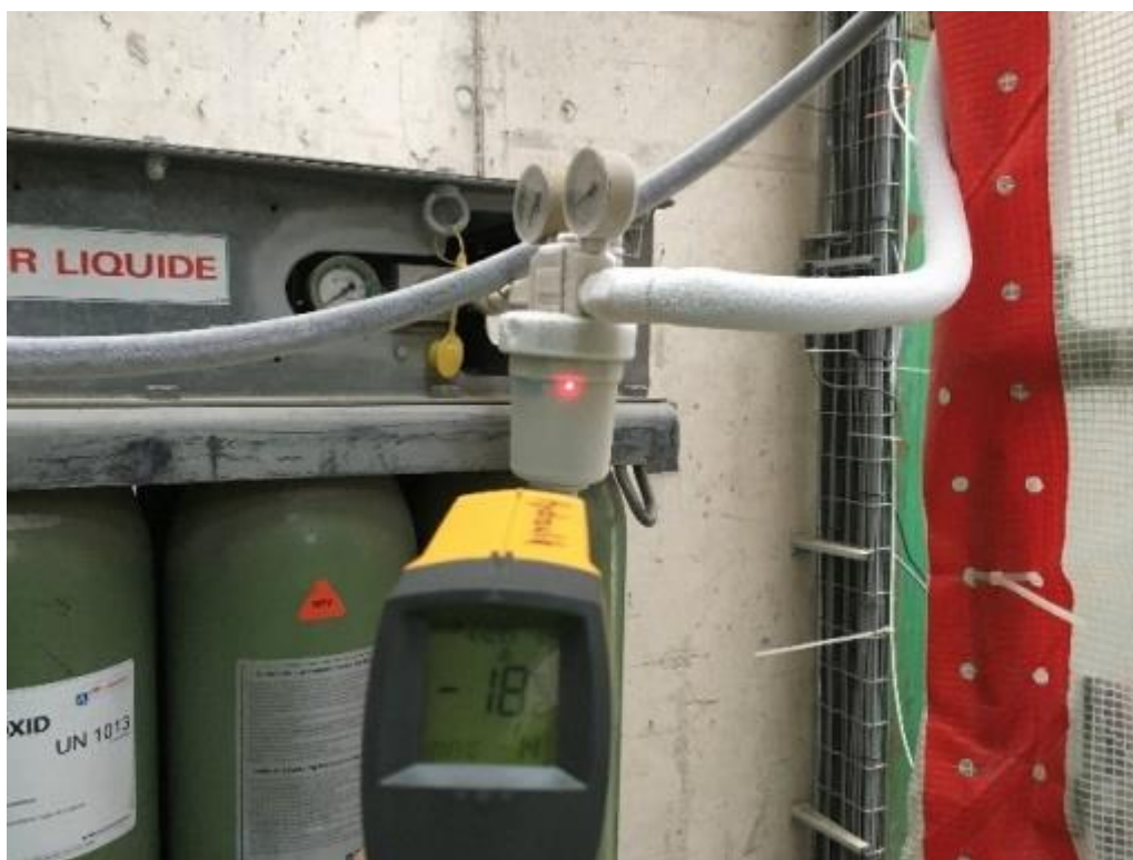
Figure 7.5: Frozen up pressure reducer of one of the CO 2 -bundles
