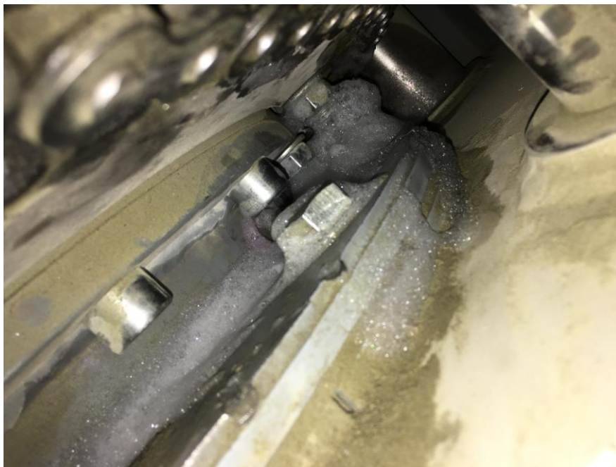
Figure 3.16: Leakage detection with soap water between rotating clinker extraction device and static pilot cooler housing
