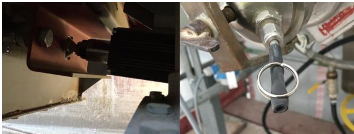
Figure 3.18: Fixed leakages observed during the tightness tests 2/2
