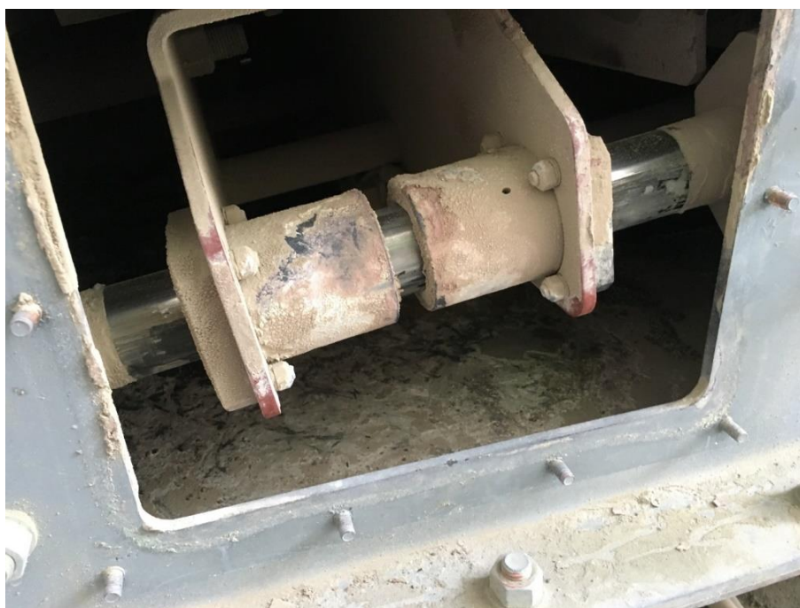
Figure 7.3: Raw meal and clinker dust clogging the linear unit of the grate suspension
