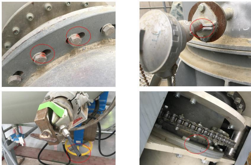
Figure 3.15: Leakages indicated by red residue from the smoke generator
