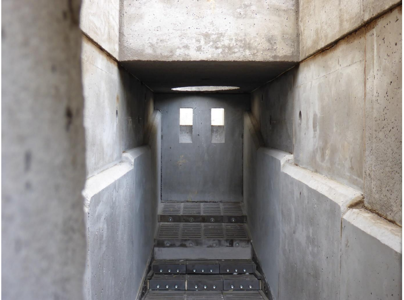
Figure 3.10: Oxyfuel clinker cooler prototype from the inside after refractory works
