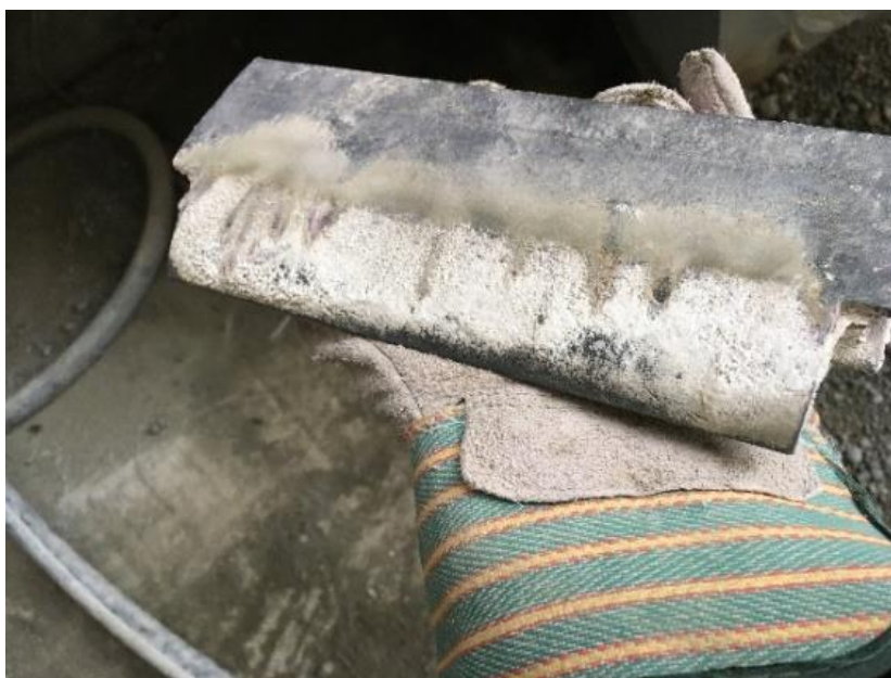
Figure 7.2: Raw meal and clinker dust clogging the lamellas of the cooler grate plates
