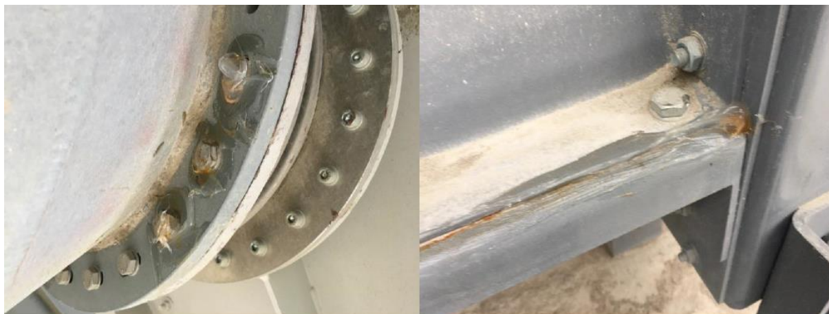
Figure 3.17: Fixed leakages observed during the tightness tests 1/2
