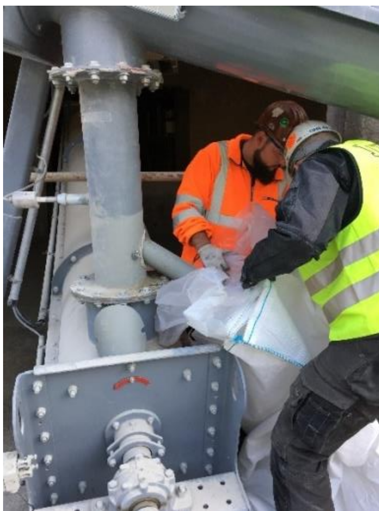
Figure 7.6: Contactless solid flow sensor and cold clinker extraction for further weighing
