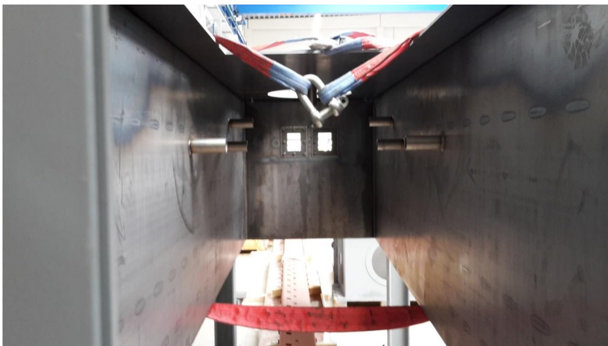
Figure 3.3: Oxyfuel clinker cooler prototype view into upper cooler housing
