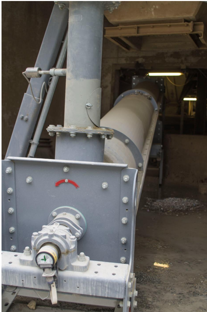
Figure 7.4: Cold clinker discharge onto the HC clinker pan conveyor
