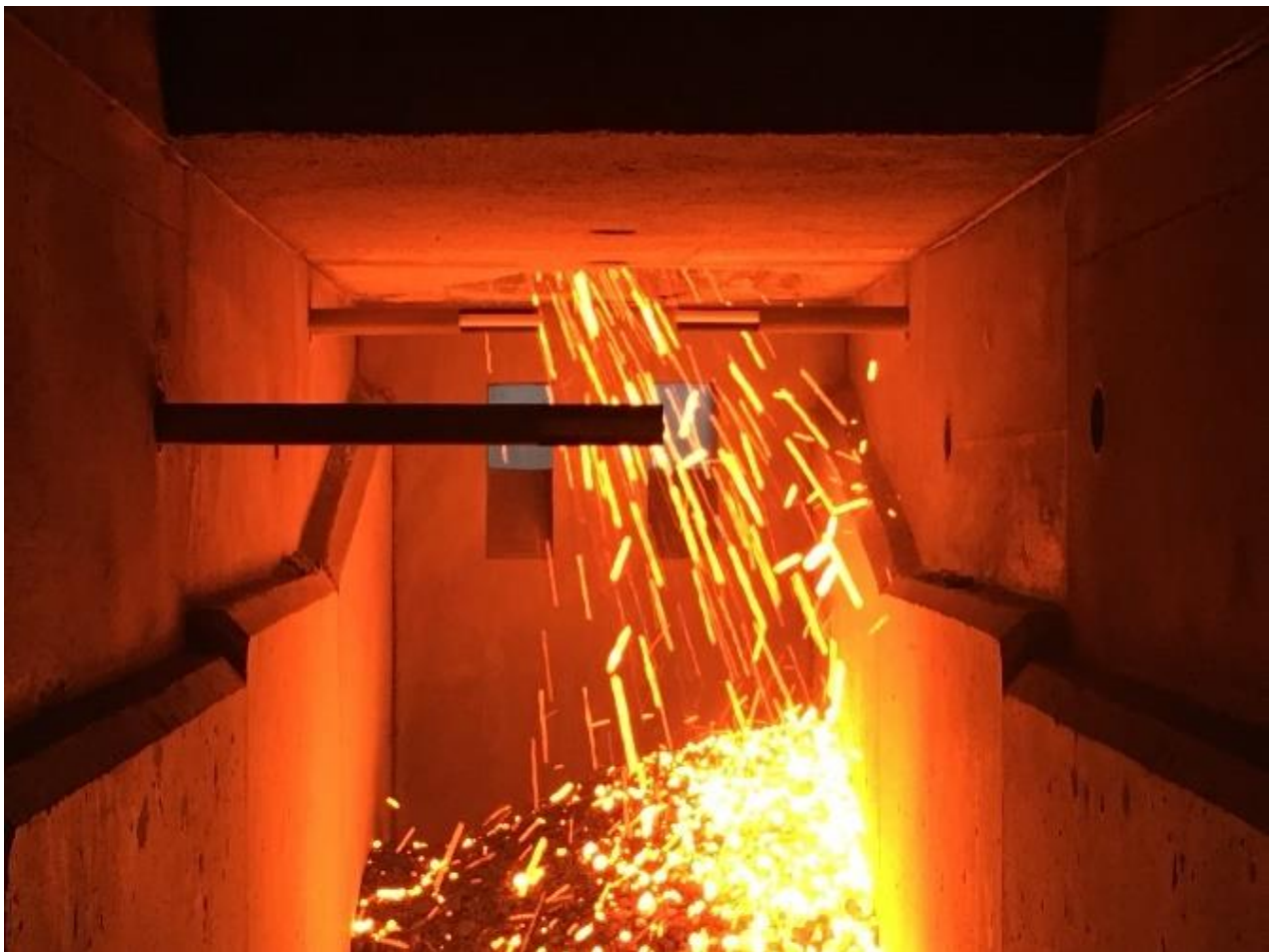
Figure 7.7: Hot clinker partially missing the static inlet section of the oxyfuel pilot cooler
