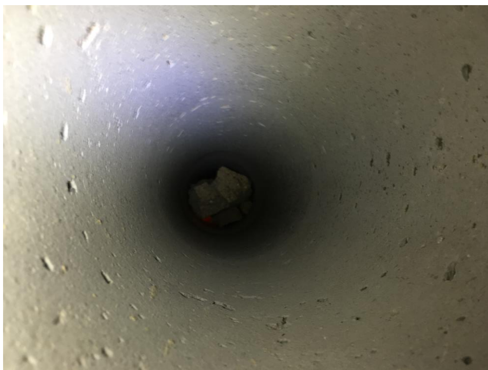
Figure 4.1: Broken refractory pieces clogging the extraction tube
