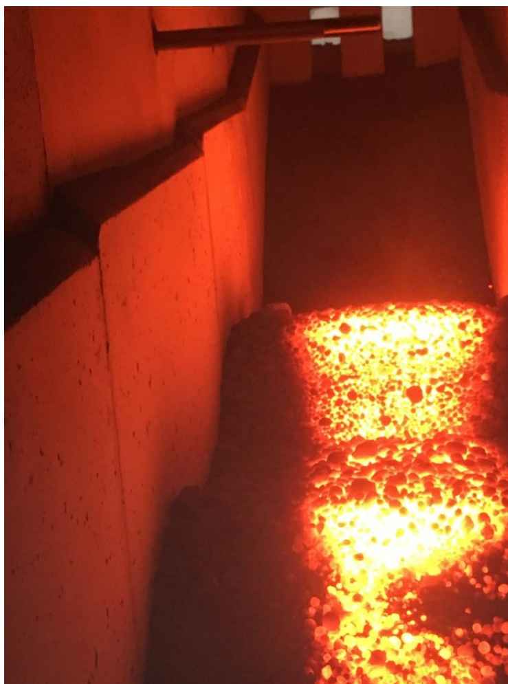
Figure 7.8: View onto the wavy clinker bed in the oxyfuel pilot cooler
