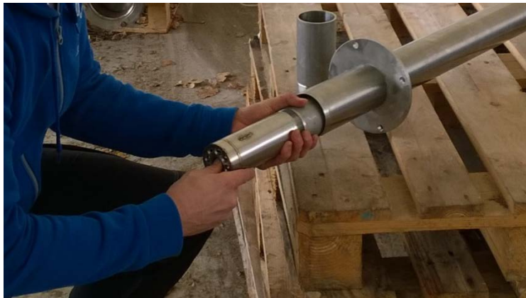
Figure 2-5: Flexibility by unmounting nozzle section in modified design.
