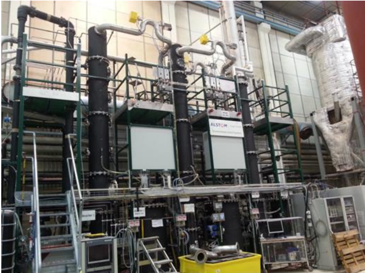
Figure 6: Test rig at Växjö used for the pilot tests of the \text{CO}_2 absorber ( \text{CO}_2 capture tests of the first experimental campaign) and the \text{NH}_3 absorber ( \text{NH}_3 removal tests of the third experimental campaign).
