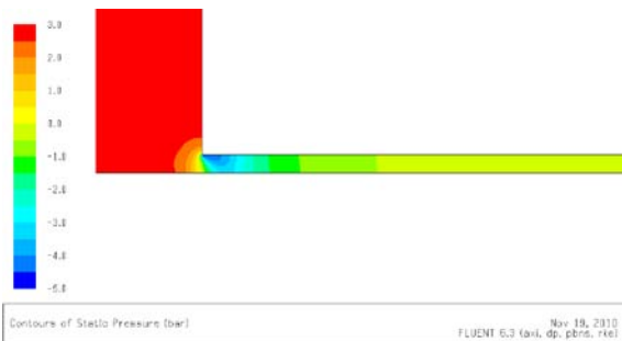
Figure 9: Pressure distribution for the C-valve, zoomed into the tight channel.
