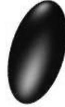
Figure 2: Super-quadric particle with aspect ratios 2:1:1 representing a rice grain.
