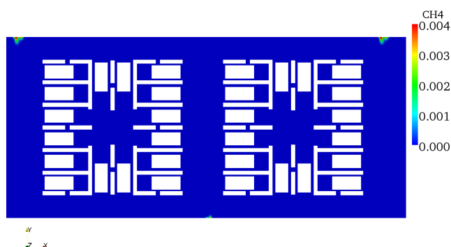
Figure 23: Molar fraction of methane (v/v) on the plane at the height of the middle of the upper burners
