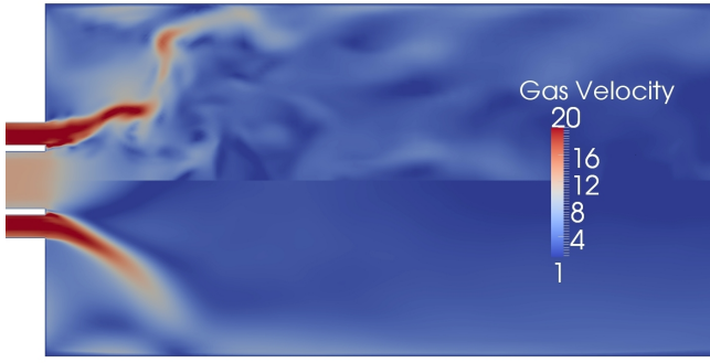
Figure 5: Instantaneous (top) and mean (bottom) contours of gas phase velocity magnitude ( m/s )
