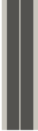
Figure 2: Model domain. The lighter area is the viscous domain, \Omega_v , representing the CSF space and the central canal. The darker area is the porous domain, \Omega_p , representing the tissue of the spinal cord.
