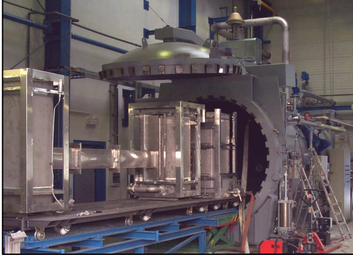
Fig. 2: TOPFLOW Hot leg model in front of the pressure chamber
