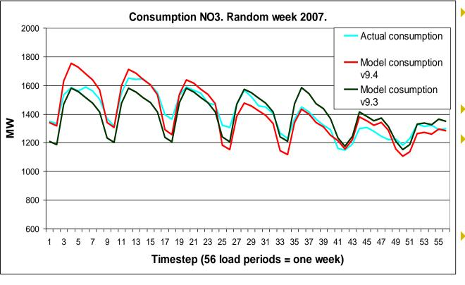
Daily temperature correction helps explain actual consumption better Still no exact match What details are most important, and where to improve model and input? The level of precision required is
