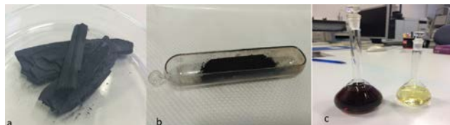
Figure 5: Biocarbon chips and powders and condensate collected from carbonization experiments
