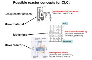
Most of the CLC demonstration work has been on circulating fluidized bed (CFB) kind of reactors. We believe that very compact reactors for CLC can be developed using rotating reactor concept. At present we are developing such a reactor – having a radially directed gas flow as shown below:
