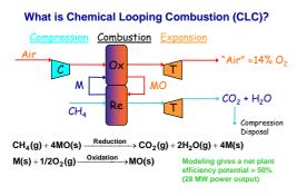
Using this technology, natural gas is combusted to pure  $\rm CO_2$  without the need for an expensive oxygen plant !
