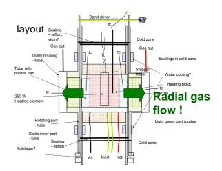
Since the oxygen carrier bed is rotating, one of the critical points is to avoid mixing of gases between the two gas streams. Below are the results from our initial experiments showing significant mixing: .
