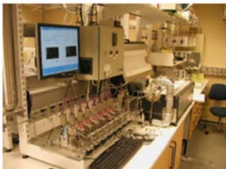
*Gas permeation unit for testing of high temperature dense hydrogen selective membranes. (Photo: SINTEF)*
