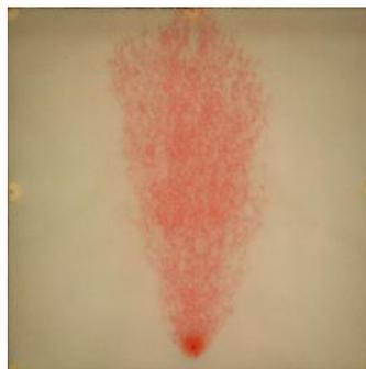
2D-cell experiment illustrating the buoyant migration of CO<sub>2</sub> in an aquifer (Polak et.al., 2010). (Photo: SINTEF)
