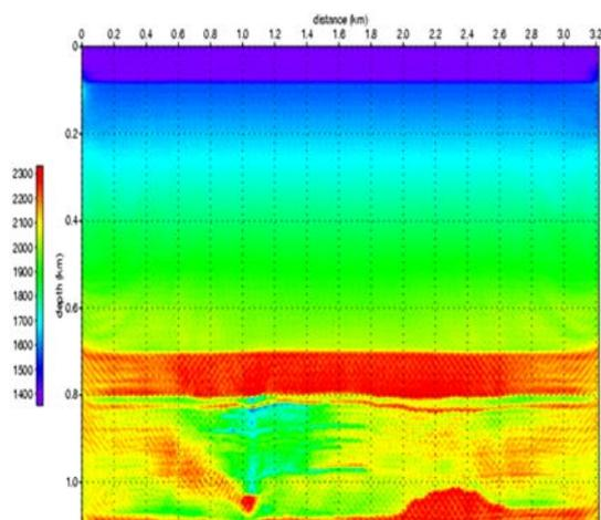
Velocity model from the Full Waveform Inversion method (Ravault et.al., 2009). (Illustration: SINTEF)
