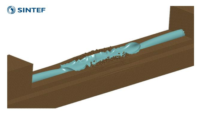
Visualization of a simulated running ductile fracture in a CO, pipeline II
