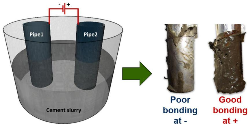
*In a SINTEF experiment, steel casing pipes with positive and negative voltage were immersed in cement slurry. This was found to strongly affect cement-steel bonding, which was improved with positive voltage. The novel concept has potential to minimize leakage paths at the cement-steel interface in wells, and thus enhance safety of CO<sub>2</sub> storage.*
