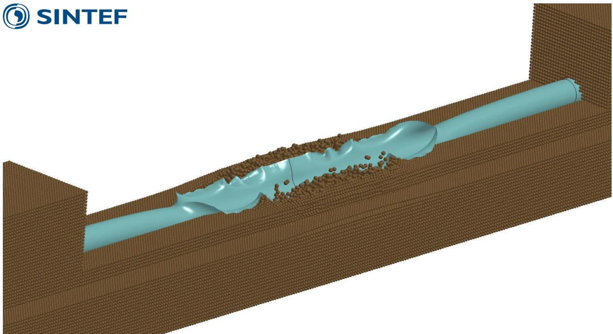
*Visualization of a simulated running ductile fracture in a CO<sub>2</sub> pipeline II*
