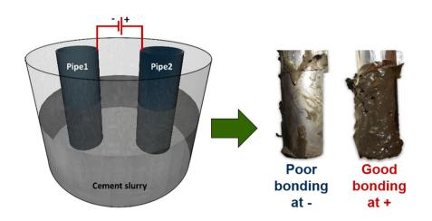
In a SINTEF experiment, steel casing pipes with positive and negative voltage were immersed in cement slurry. This was found to strongly affect cement-steel bonding, which was improved with positive voltage. The novel concept has potential to minimize leakage paths at the cement-steel interface in wells, and thus enhance safety of CO<sub>2</sub> storage.
