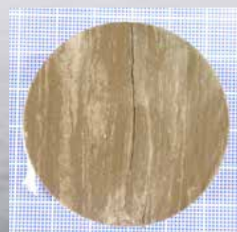
Figure 2: Tensile testing with compression perpendicular and along bedding planes to the well axis.
