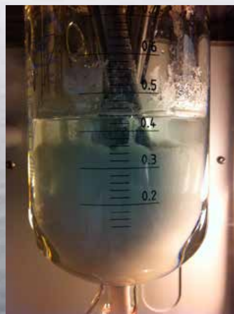
Pictorial illustration of precipitation at process condition upon CO 2 absorption
