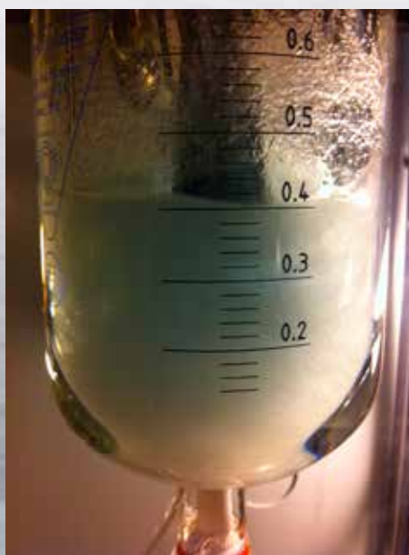
Pictorial illustration of precipitation at process condition upon CO 2 absorption
