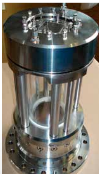
New improved optically accessible oxy-fuel combustor of the HIPROX facility.
