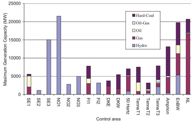
Figure 4: Installed regulating generation capacity in each sub-area.
