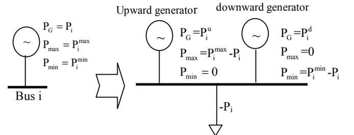
Fig. 2. Generators represented in IDC-OPF
