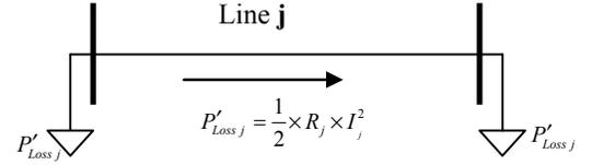
Fig. 1. Loss represented as loads at both ends of transmission line
