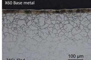
Figure 1: Micrographs of the interface microstructure. Left: Sample A, Right: Sample B.
