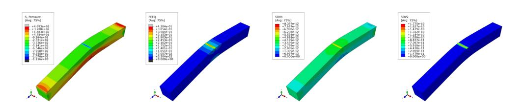
Figure 7: FE simulation for verification of the hydrogen transport model implementation: encastred beam subjected to thermo-mechanical boundary conditions. From left: 1) Hydrostatic pressure (p [MPa]), 2) Equivalent plastic strain ( $\varepsilon_{p}$ ), 3) Lattice hydrogen concentration ( $C_{L}$  [mol/mm<sup>3</sup>]), 4) Trapped hydrogen concentration ( $C_{\tau}$ [mol/mm<sup>3</sup>]).
