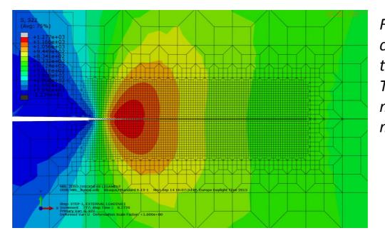
*Figure 8: Stress distribution in a 2D MBL* cohesive zone model of a growing crack at the interface between clad and base metal. The upper part of the model is the base metal while the lower part is the clad material.
