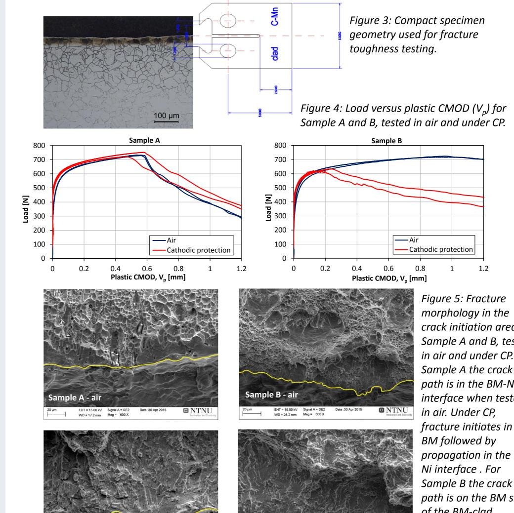
crack initiation area. Sample A and B, tested in air and under CP. For Sample A the crack path is in the BM-Ni interface when tested fracture initiates in the propagation in the BM-
