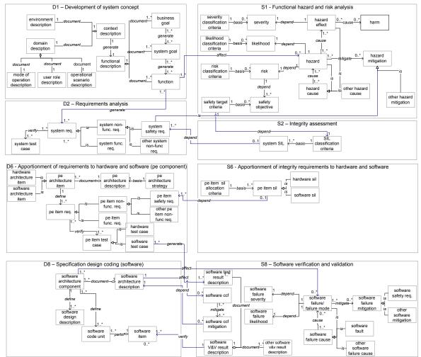
Figure 5 Applicable levels of traceability process model for SafeScrum
