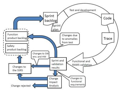
Figure 4 SafeScrum extended with the IEC 60880 change impact analysis
