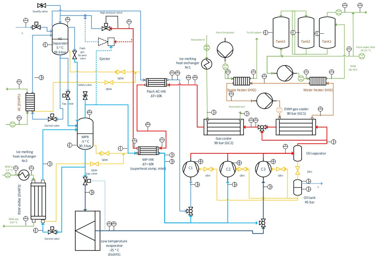
Figure 1: Principal sketch of the transcritical CO<sub>2</sub> refrigeration system
