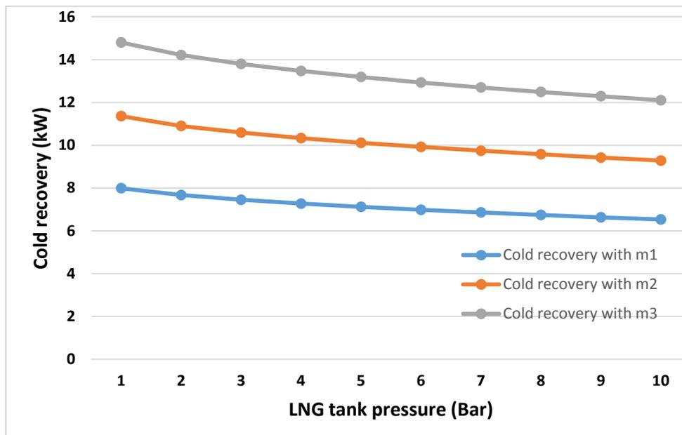
**Figure 5: LNG tank pressure versus cold recovery potential**
