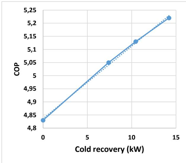
Figure 2a: LNG cold recovery versus COP
