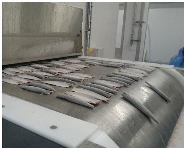
Figure 3: Combined blast and contact freezing of mackerel filets
