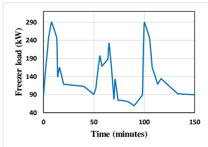
Figure 1b: Freezing load profile
