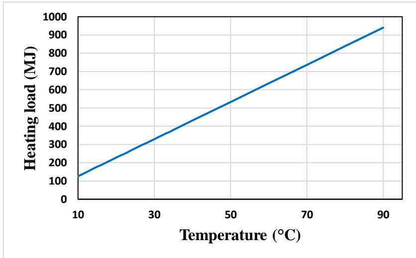
Figure 2: Heating demand for RRM thermal treatment
