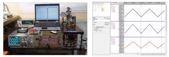
Set-up for innovative interfacial contact resistance measurements (ICR), developed at UPT, Romania
