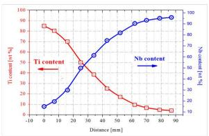
Compositional spread in the Ti-Nb system manufactured by magnetron sputtering out of elemental targets
