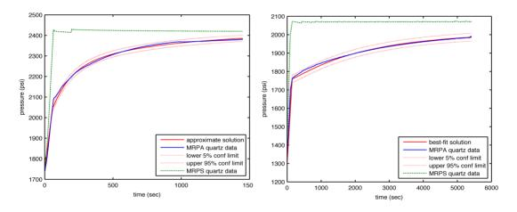
Figure 3 Best-fit model results to VIT data from the TPX (left) and CC1 (right) wells. Shown are the measured MRPA data in blue and the model results obtained from parameter estimation in red. The uncertainty of the best-fit solution is tied to the PDF of estimated wellbore permeability values produced by the parameter estimation algorithm [11]. The 95% confidence in the best-fit solution is bracketed by the dotted red lines.
