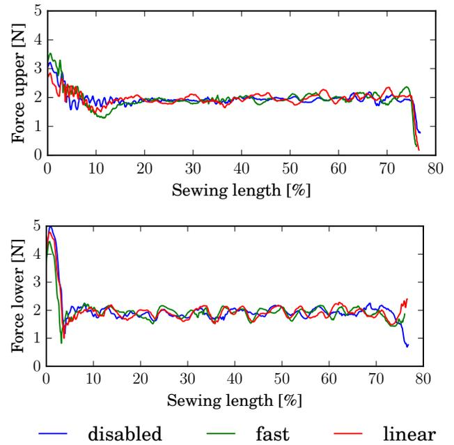
Fig. 10. Sewing forces for sewing of parts with different edge lengths with different strategies.
