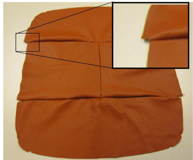
Fig. 6. Without velocity synchronization, the corners of the two parts are not ensured to match.
