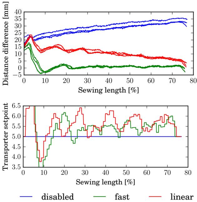
Fig. 9. Distance differences and transporter setpoints for sewing of parts with different edge lengths with different strategies.
