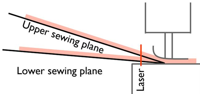
Fig. 4. Different virtual sewing planes are used for the two robots to prevent collisions and to ensure that the parts can move freely.
