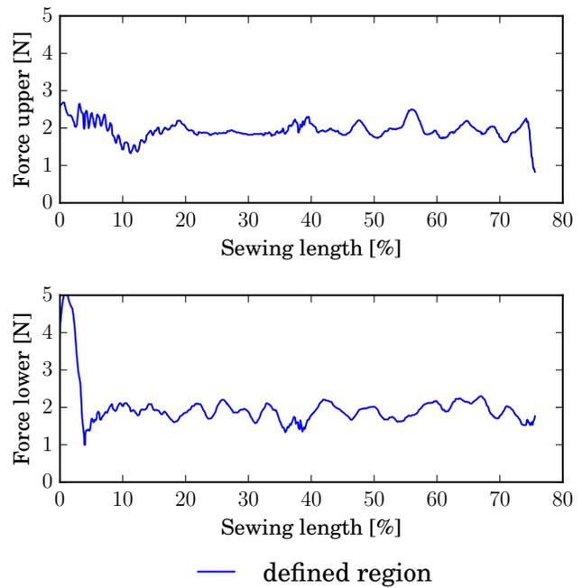
Fig. 12. Sewing forces for sewing of parts with different edge lengths. The initial error is compensated in a defined region, between 30 and 60 % of the seam.
