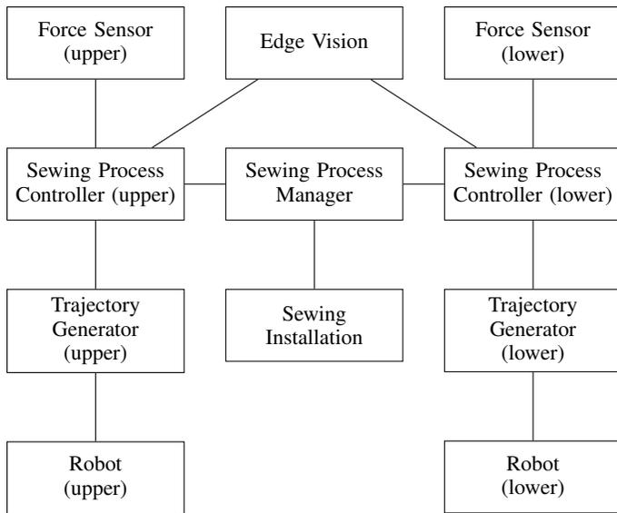
Fig. 3. Overview of the components in the system.
