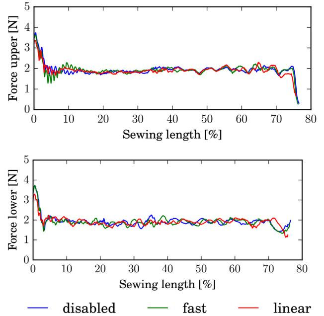
Fig. 8. Sewing forces for sewing of two similar parts with different strategies.
