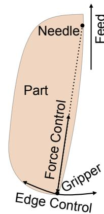
Fig. 5. The control concept of the robot for edge and force control. The two controllers work independently.
