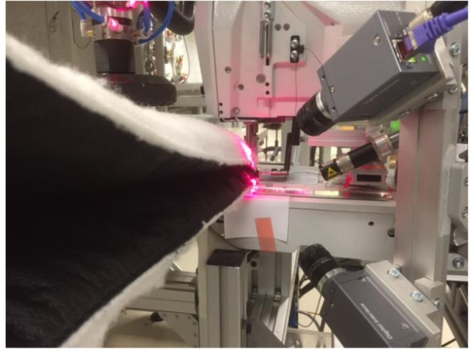
Fig. 2. The edge sensor system consists of two cameras and a laser that projects a laser line directly on the lower part. A mirror is used to project the laser line on the upper part.
