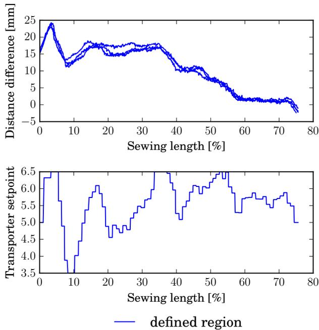
Fig. 11. Distance differences and transporter setpoints for sewing of parts with different edge lengths. The initial error is compensated in a defined region, between 30 and 60 % of the seam.
