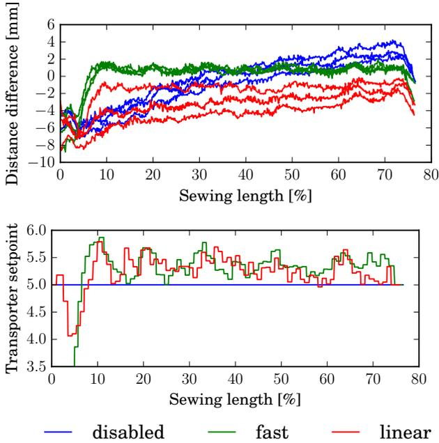
Fig. 7. Distance differences and transporter setpoints for sewing of two similar parts with different strategies.
