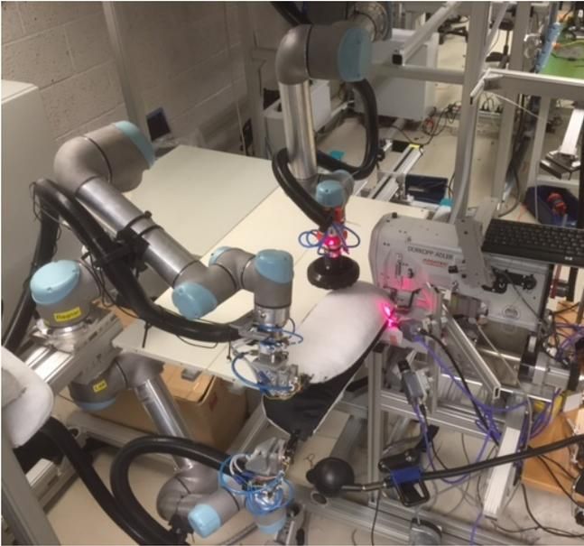
Fig. 1. The sewing cell demonstrator consists of a sewing machine and three robots that handle the parts during the sewing operation. Sensor systems are installed to measure the force in the parts and the edge position in front of the needle.
