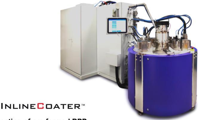
Coating of pre-formed BPP Both sides simultaneously
