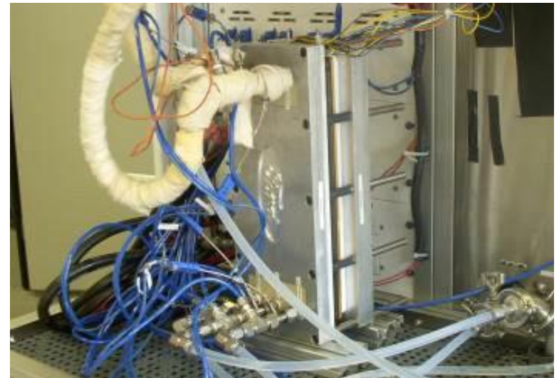
Ford short stack with TreadStone metal bipolar plates
