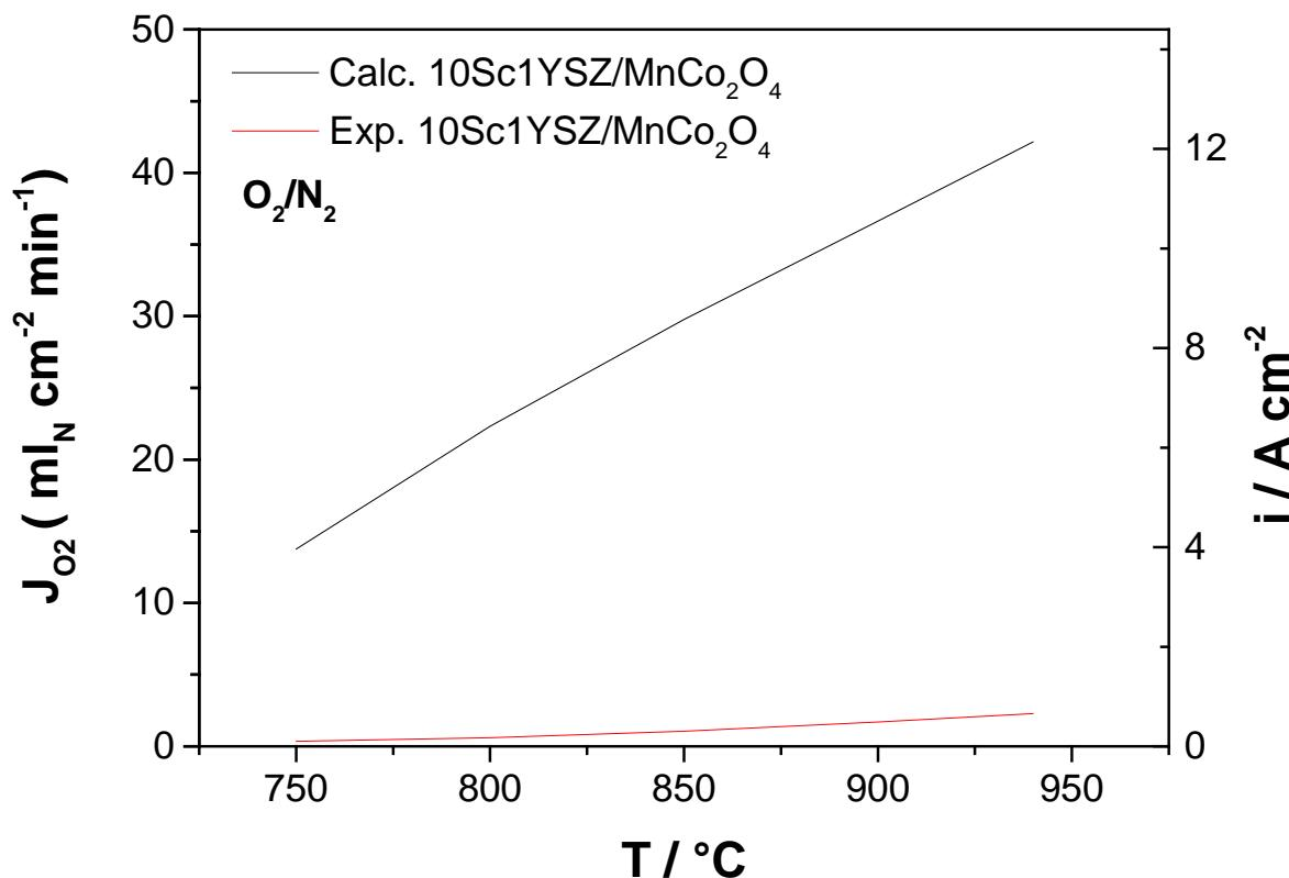
$$i = \frac{RT}{4F} \frac{(\alpha \sigma_{ion,ScSYZ} + \beta \sigma_{ion,MCO})}{t} \ln\left(\frac{p'}{p''}\right)$$
