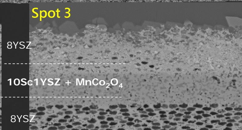
Oxygen flux through ScYSZ- $\text{MnCo}_2\text{O}_4$  (70-30 vol.%) membranes could be ~2 times higher without the impurities from the sealing material!
