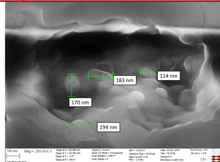
Particles size 4 times higher after test =  $\searrow$  surface area = degradation catalysts activity
