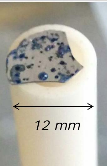
Membrane's picture after test (Anode side  $\text{CO}_2/\text{N}_2$ )
