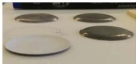
❖ Two-step sintering → Successful development of dual phase 10Sc1YSZ/MnCo<sub>2</sub>O<sub>4</sub> asymmetric membranes
