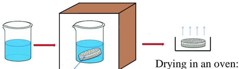
Immersion membrane in aqueous solution **3 min** in vacuum chamber
