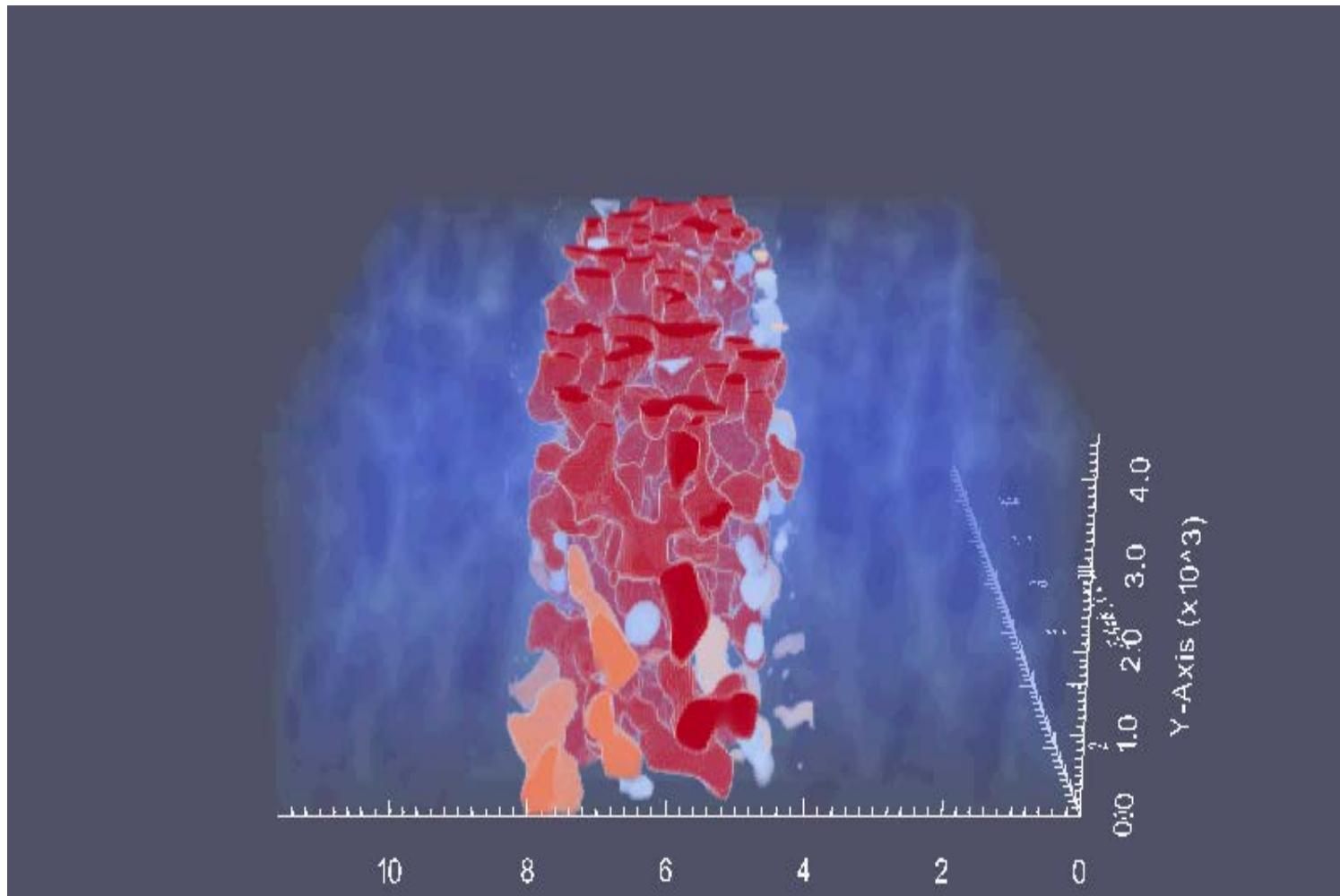
90 % of the MCO grains are connected to both sides of the dual-phase layer.
