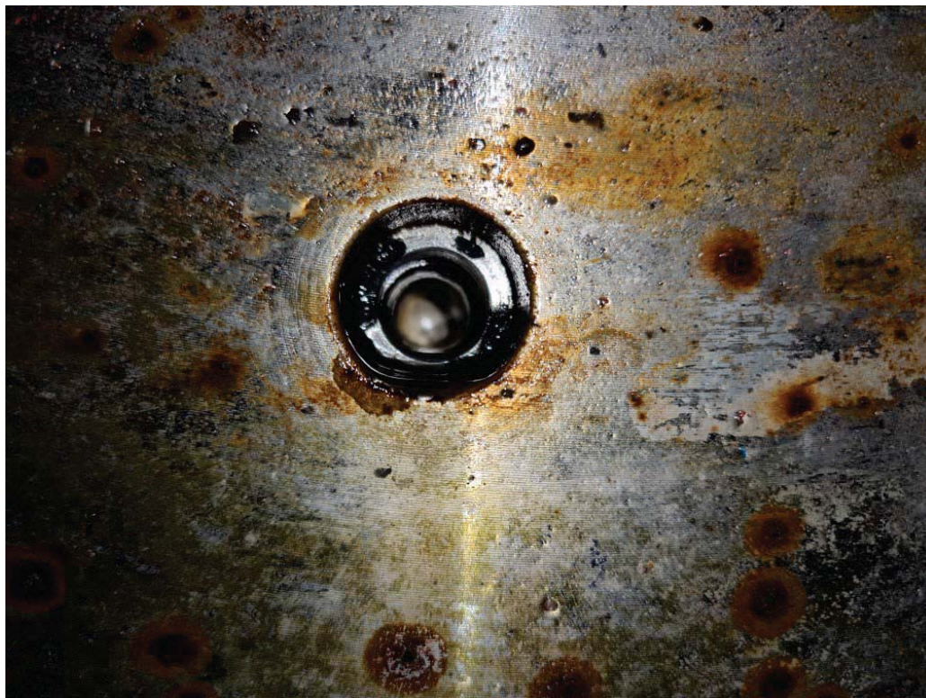
Figur 12. Korrodert skrueshull i kapsel for propellhode
