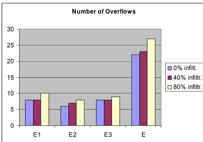
**Figure 16: Number of overflows of 3 CSO structures and sum of overflows**
