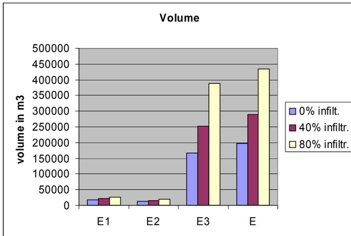
**Figure 15: Discharged volume of 3 CSO structures and total volume**
