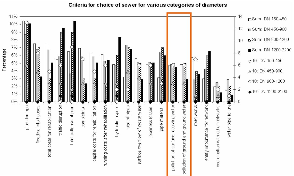
**Figure 1: Decision criteria for sewer rehabilitation (CARE-S Deliverable D16)**
