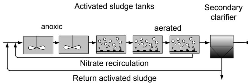
**Figure 6: scheme of the WWTP**
