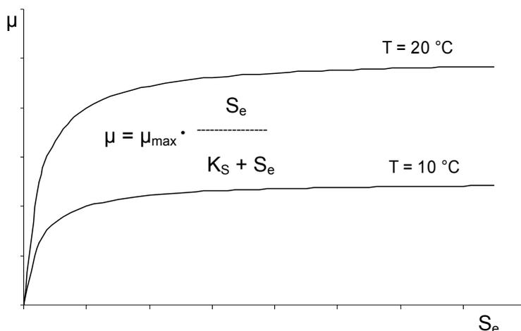
Figure 5: Influence of temperature on Monod relation (after Kroiss and Prendl, 1996)
