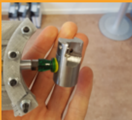
A vacuum gripper will be used in the physical experiment. By using a differential flow sensor it is possible to distinguish a successful from an unsuccessful grasp.
