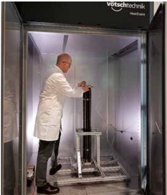
Installation of cement plug prior to temperature and pressure exposure.
