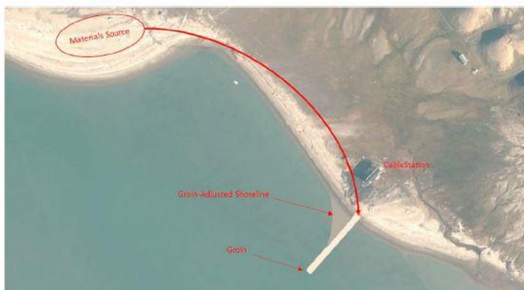
Figure 94. Groin for Hiorthhamn, Photo: © TopoSvalbard, figure: from [31].
