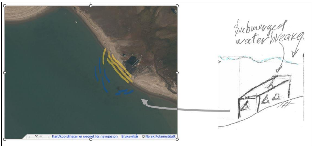
Figure 93. Temporal protection (geotextile bags) combined with submerged breakwater.
