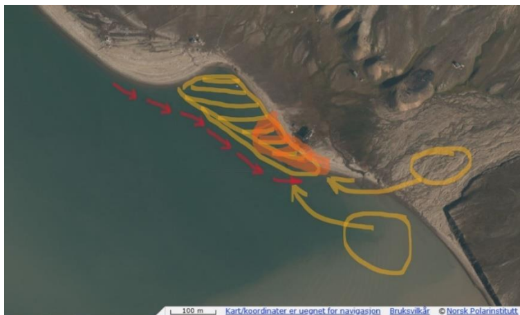
Figure 95. Principal scheme for artificial beach. Photo: © TopoSvalbard.
