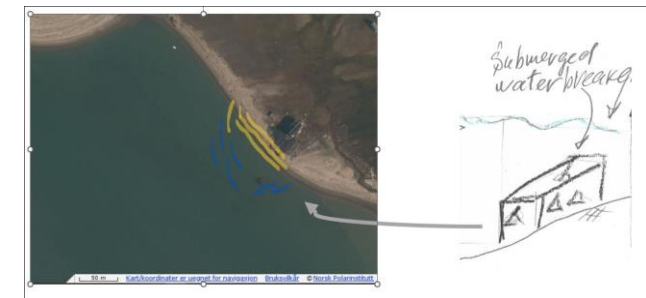
Figure 1. Temporal protection (geotextile bags) combined with submerged breakwater.
