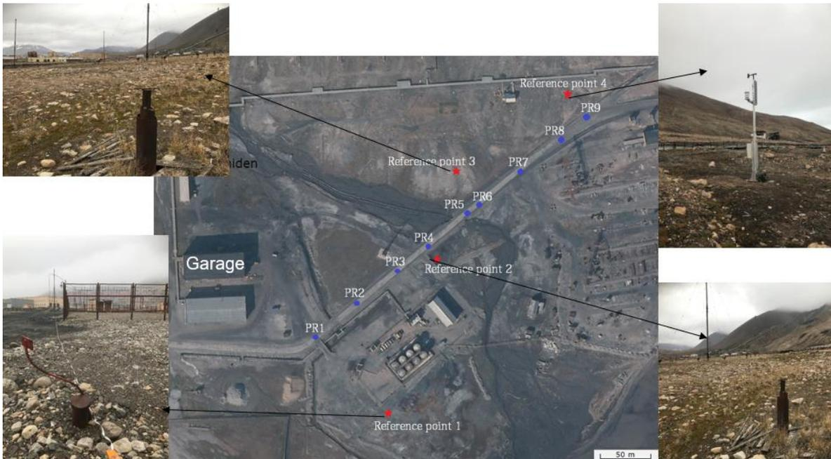
**Figure 4. Locations of the monitoring objects in Pyramiden: the multi-purpose garage, reference points, and monitoring points on the road (PR1–PR9).**
