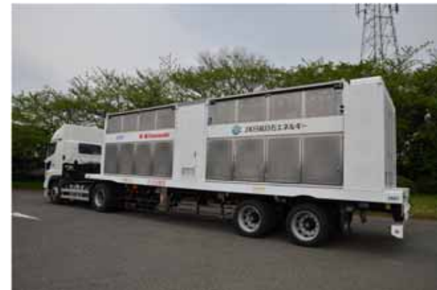
High pressure hydrogen gas trailer
