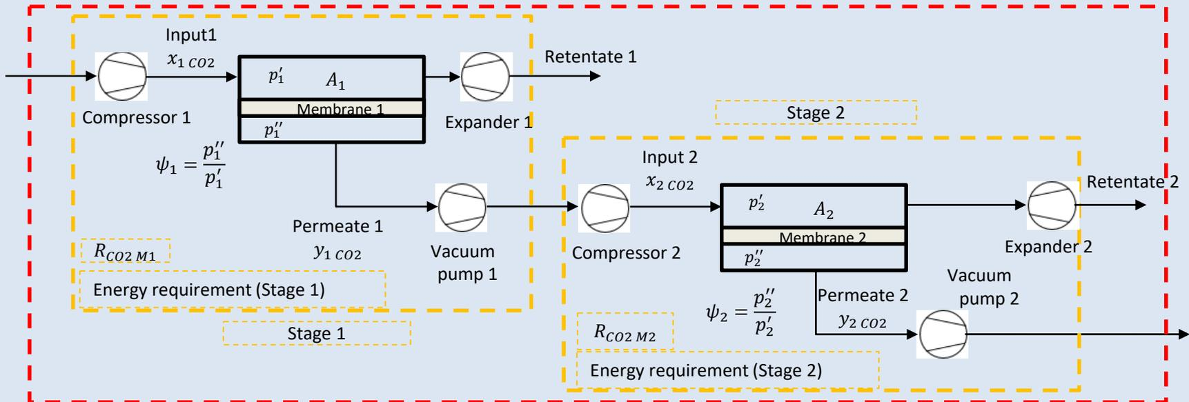
Two-stage membrane process is needed to attain the specification in term of CO<sub>2</sub> purity and recovery
