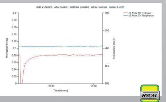
Close Step 8 - Measurement complete H = 0.079[ml/100a] H Span = 0.007[m]/100g] Allov = Custom T = 705.0[C]Melt code = Custom T Span = 1.2[C] Lot No = Example Analysis time = 5[minutes] Worker = A Smith Measurement finish time = 21/12/2015 15:31:03 Measurement: 1 of 1
