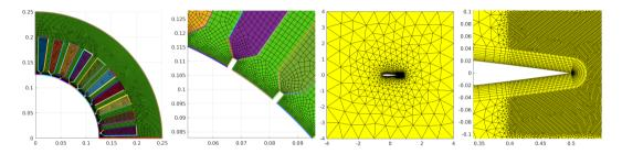
*Left*: A quarter of a stator with multiple labelled subdomains and labelled edges. *Right*: A NACA 12 airfoil modelled by a triangular/quadrilateral grid with boundary layer.
