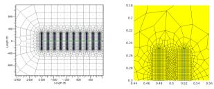
Left: Mesh from KAPPA with multiple structured boundary layers (figure from Artus, Fructus. OGST 67(5)). Right: Similar example using Gmsh with automatic boundary layer <sup>5/8</sup>and fan around two 1D fractures.
