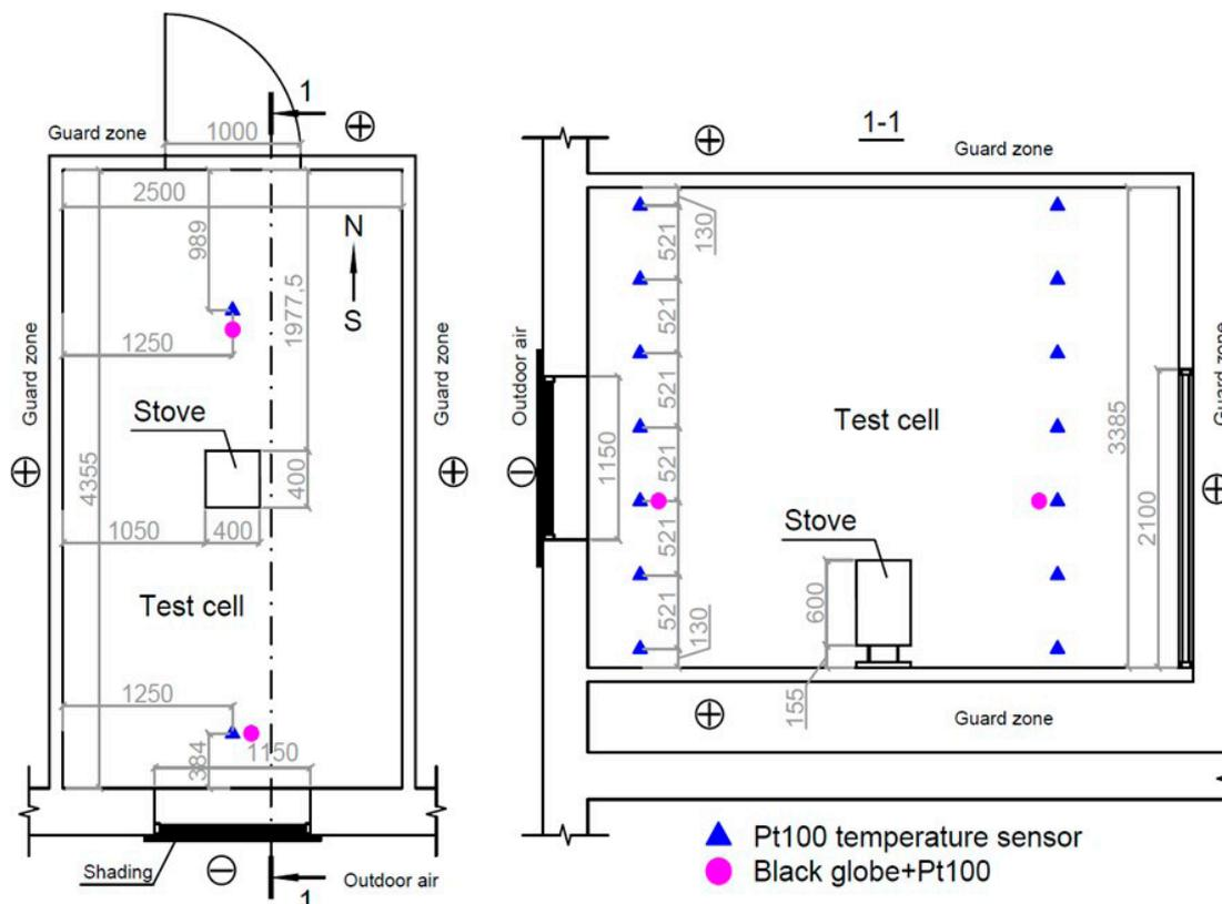
Sketch of a laboratory room in Trondheim heated using an electric stove that mimics the heat emission of real wood stoves: the measured air and wall temperatures are compared to simulations
