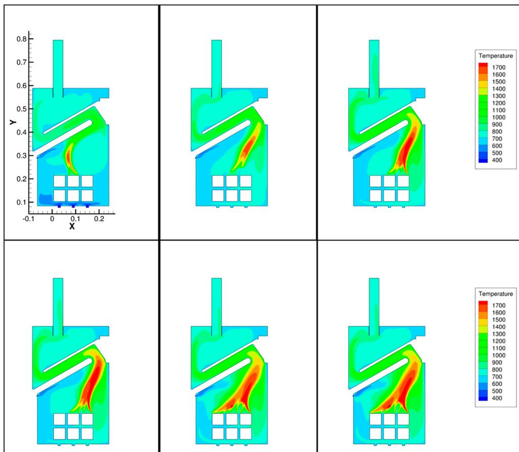
Temperature (K) at different time during the wood combustion cycle [1]
