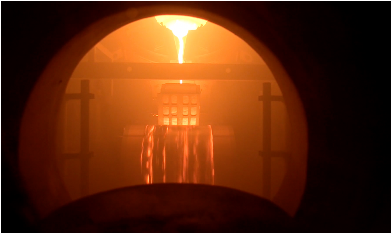
Inside of one of the 600kg strip casters. Molten alloy is cast over a water-cooled rotating wheel to give flake product.
