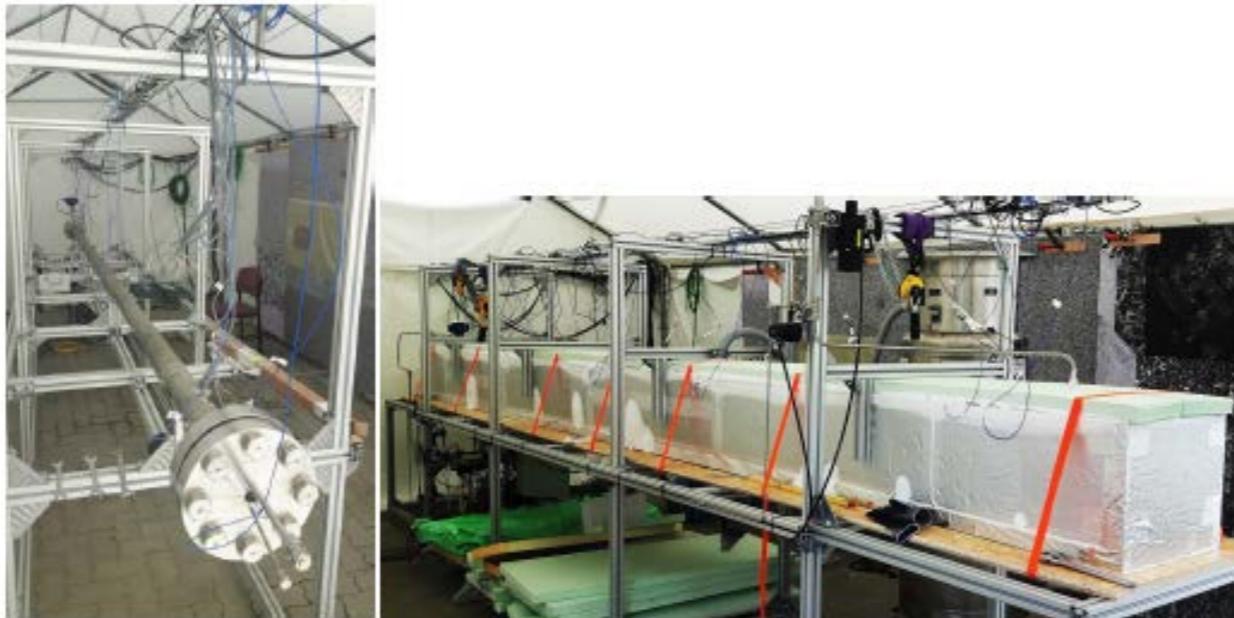
KIT/PS E5.2 cryotube FA and DDT experiments
