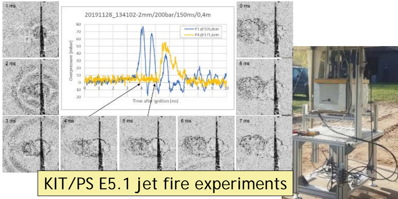
> 100 Ignited jet tests combined with discharge experiments E5.1
