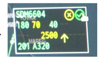
The recognized **commands are prefilled** in the **radar label** in yellow and if they are **not rejected within 10 seconds** they turn to normal green colour. The command are already shown during ATCO is still speaking. ASR integrated in the CWP: Voice commands supporting situational awarness during sectorization changes
