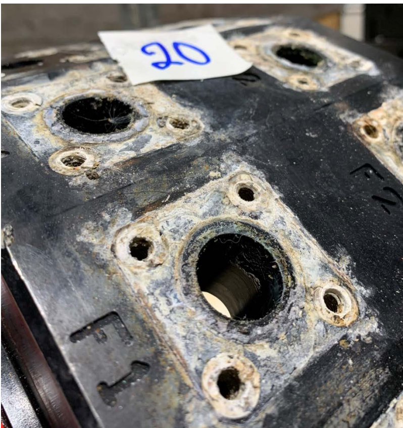
Figure 13. Crevice corrosion on anodized aluminium inside crevice against stainless steel.
