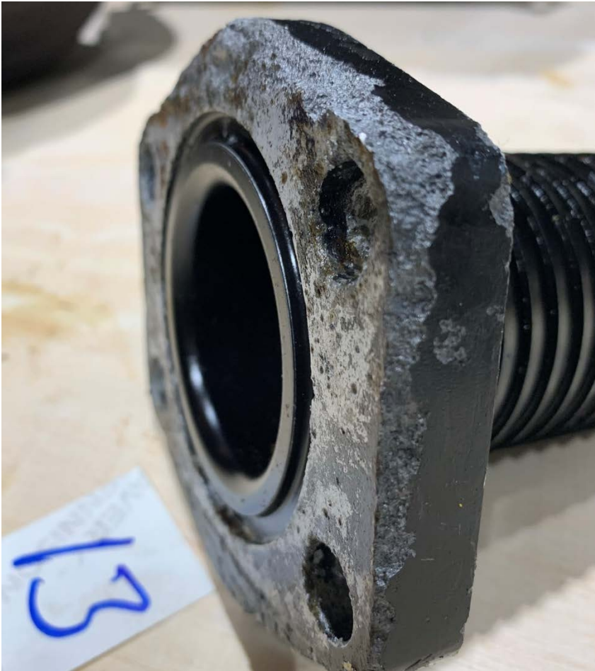
Figure 15. Severe galvanic corrosion on anodized aluminium.
