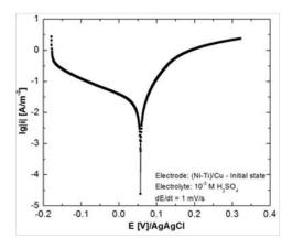
Linear polarization curves (Tafel plots) on (Ni-Ti)/Cu electrode in H2SO4 10-3 M + 0.1 ppm F-1 at room temperature recorded at 1mV/s scan rate.
