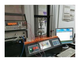
Set-up in UPT ICR measurement
