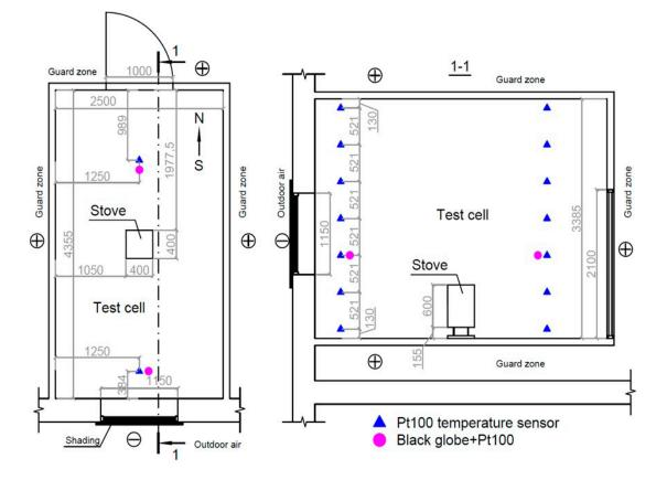
Sketch of a laboratory room in Trondheim heated using an electric stove that mimics the heat emission of real wood stoves: the measured air and wall temperatures are compared to simulations
