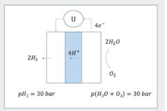
Proton ceramic electrolysers have the benefit of a high pressure of high purity hydrogen balanced with the sum of steam and oxygen.
