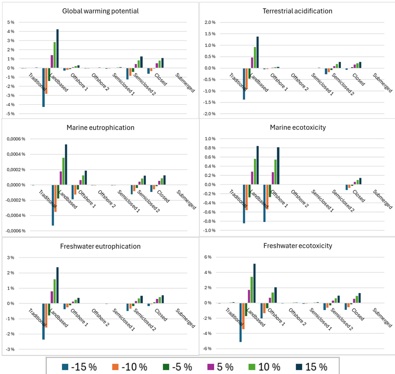
Figure 16: Sensitivity of the total footprint when changing the electricity use with -15%, -10%, -5%, +5%, +10%, and +15%. The changes in total footprint per category are represented as the percentage change to the baseline result which are presented in sections 3.2 -3.7.
