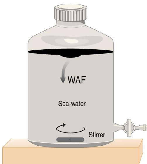
Figure 1. System for preparation of WAF
