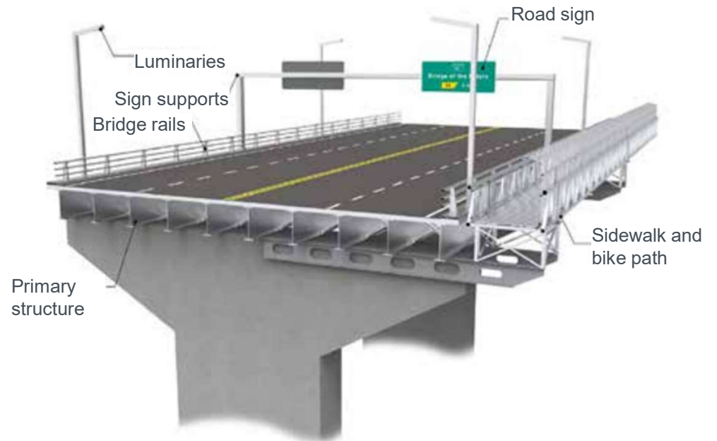
Cross section of a road bridge with aluminium superstructure and secondary components (MAADI Group).
