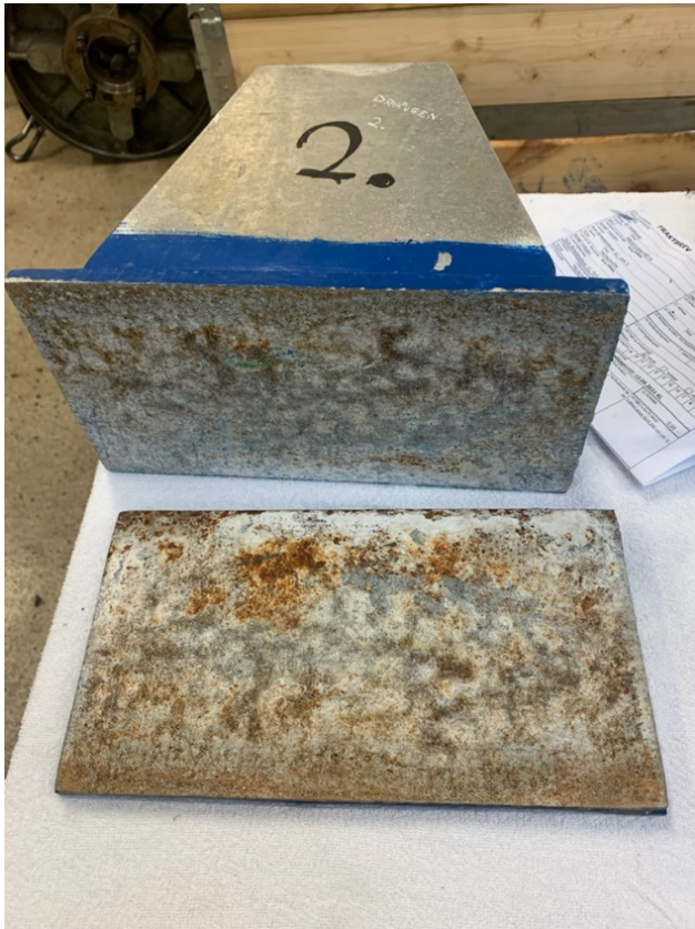
Fracture along the weld interface
