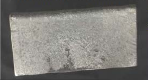
Extruded tube from permanent immersion zone
